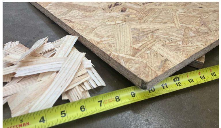
Figure 17. Tree logs are processed into veneers and flakes to make plywood and OSB.
