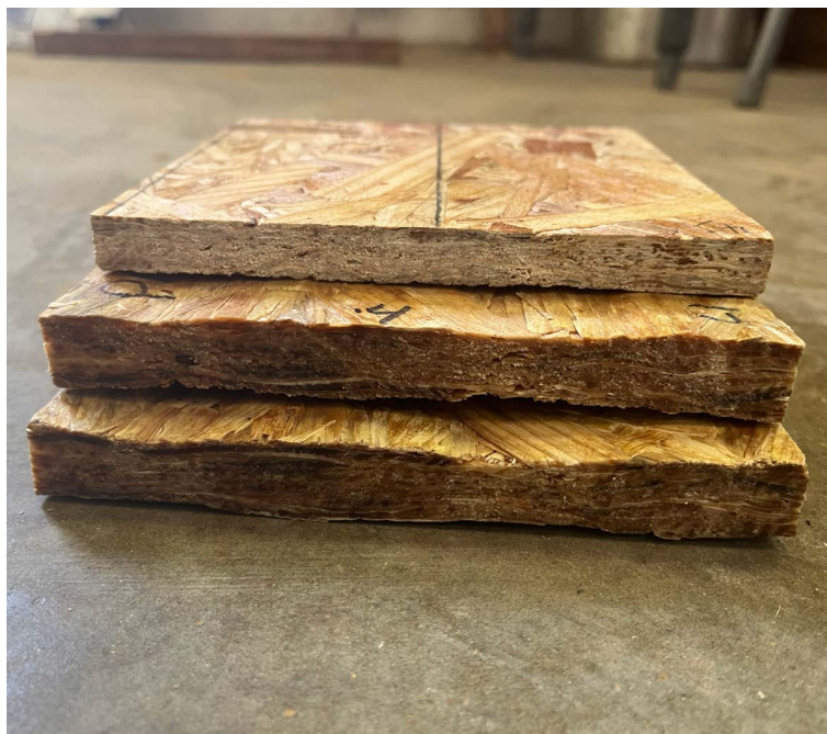
Figure 30. Thickness swelling of oriented strand board (OSB) after water absorption.
