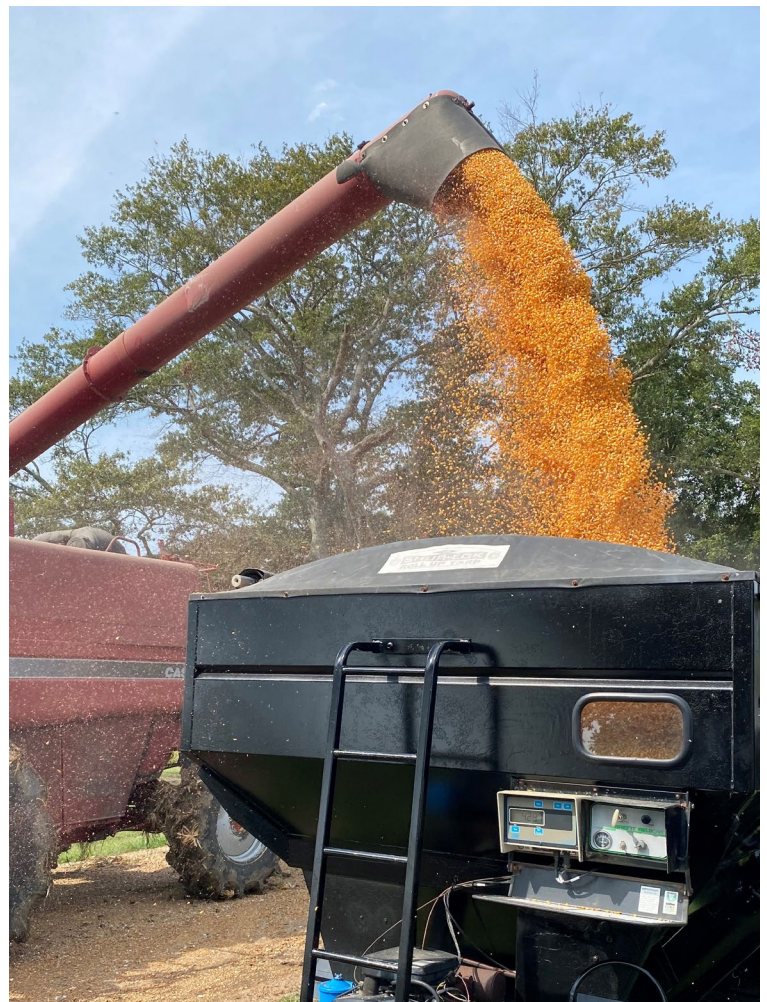
Figure 2. A combine unloads into a weigh cart as part of the calibration process.
