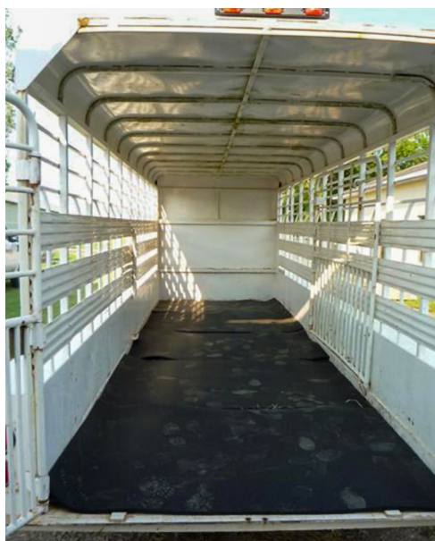
Figure 2. Rubber mats improve traction on trailer flooring.
