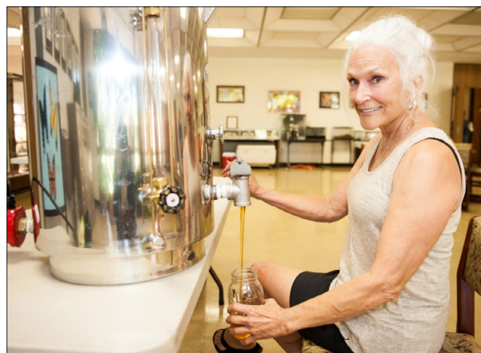
Figure 6. Jill Phillips bottles honey from a 15-gallon bottling tank that MSU Apiculture uses to heat honey at 135°F for an hour to kill the yeast.
