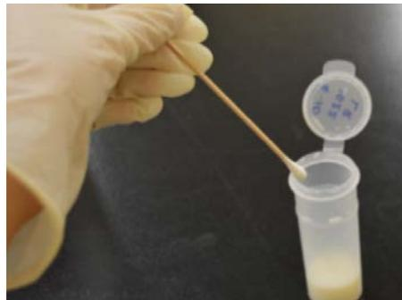
5. Re-dip the swab in the milk vial, and repeat step 4 for the remaining agar sections. The same swab can be used for all three agar sections, but discard it after all three sections are streaked.
