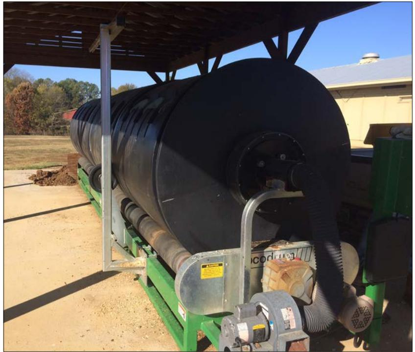
Figure 1. Ecodrum™ rotary drum composter.
