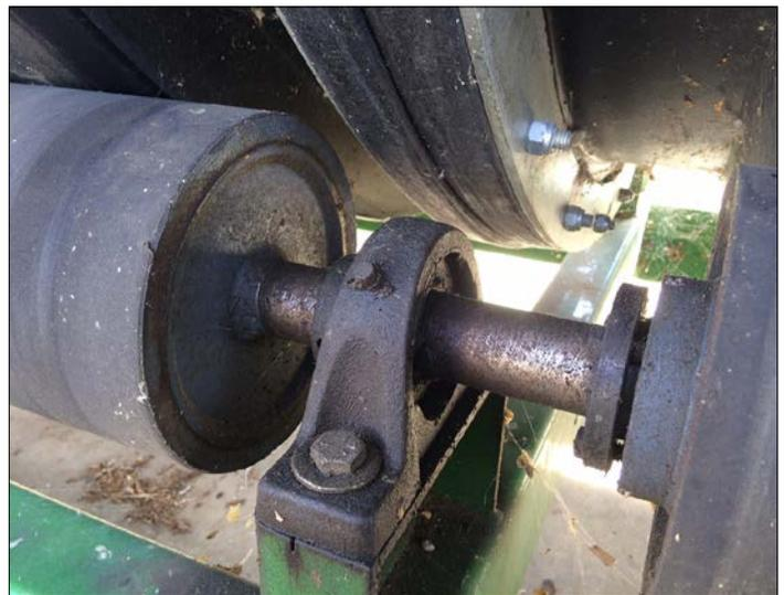
Figure 9. Grease fittings should be greased every quarter.
