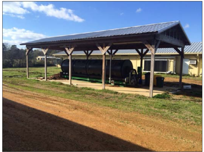
Figure 1. Rotary drum composter.
