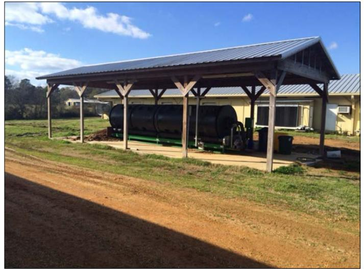
Figure 1. Rotary drum composter.
