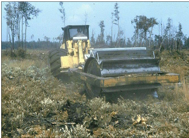
Figure 4. Smaller residuals are cut into pieces by a rolling drum chopper. The drum can be filled with water to add weight.
