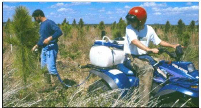
Figure 8. Advances in application technology for herbicides include smaller spray rigs for all-terrain vehicles.
