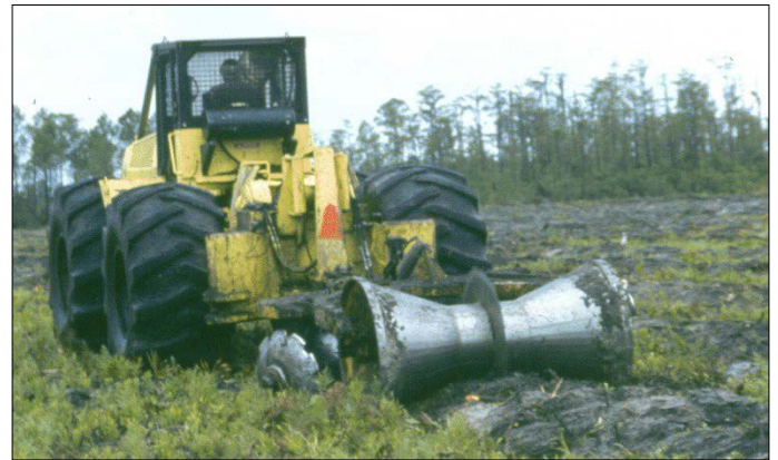
Figure 6. The bedding harrow cuts and mounds the soil into a planting row for enhanced drainage on wet sites.
