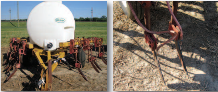
A Coulter rig or knife rig is the most cost-effective and user-friendly way to apply nitrogen to row crops.
