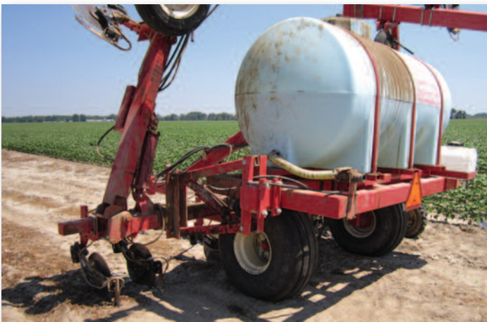
A Coulter rig or knife rig is the most cost-effective and user-friendly way to apply nitrogen to row crops.
