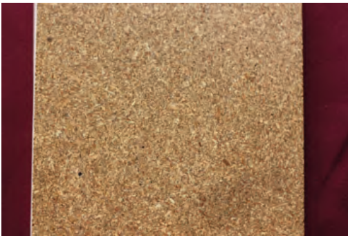
Image 5. The end of a piece of particle board; notice the individual particles.
