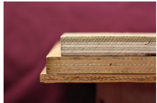
Image 3. The layers of three different thicknesses of plywood.
