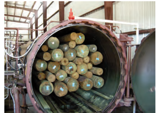
Image 2. Poles in a treating cylinder after being treated with a chemical.
