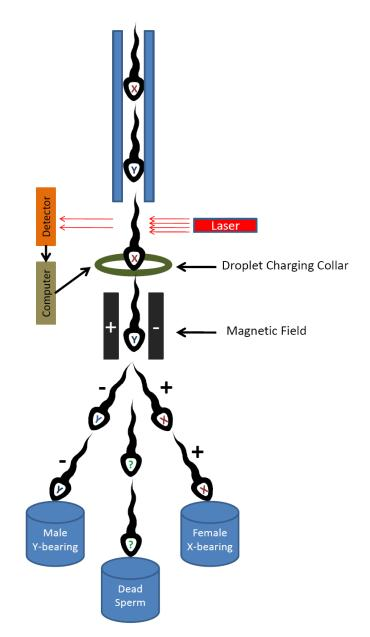
Figure 1. Schematic of flow cytomtry to sort X-bearing and Y-bearing bovine sperm cells.
