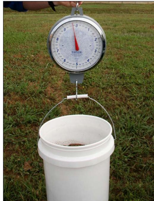
**Step 6.** Weigh the bucket and litter (or bucket, tarp, and litter). Record the empty weight of the bucket before collecting the litter on the tarp. Subtract the weight of the empty bucket to calculate the weight of the litter material applied. Do this for each of the four middle tarps. For example, the bucket and the litter in the picture weigh 9.75 pounds, and the empty bucket weighs 1.75 pounds. So the litter applied to the tarp weighs 8 pounds.
