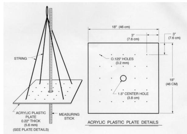
Figure 2. Falling plate meter schematic (Rayburn and Lozier, 2003.)
