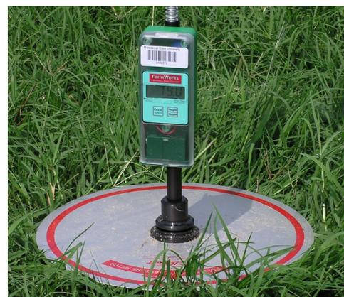
Figure 3. The falling/rising plate meter for estimating available forage in a pasture.
