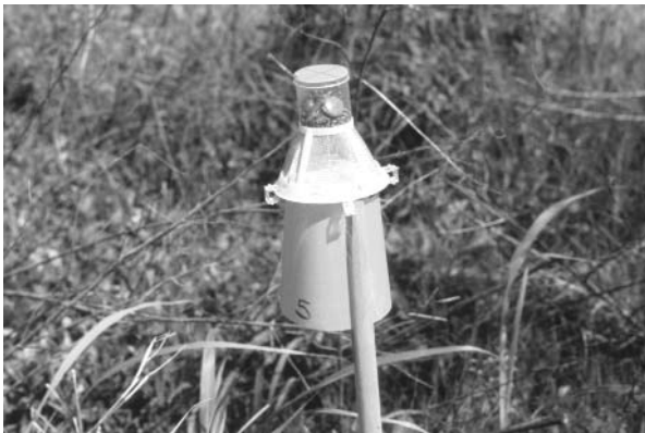
Figure 1. Boll weevil pheromone traps are memorial monuments to one of Mississippi's most important insect pests. Without the pheromone trap, it would have been impossible to eradicate the boll weevil. Pheromone traps are also the most important tool for detecting boll weevil reinfestations. Consequently, Mississippi cotton growers should take care to avoid damaging traps that are being run in their fields.
