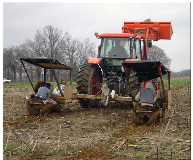
Figure 7. Artificial regeneration of shortleaf pines showing machine planting of retired cropland.
