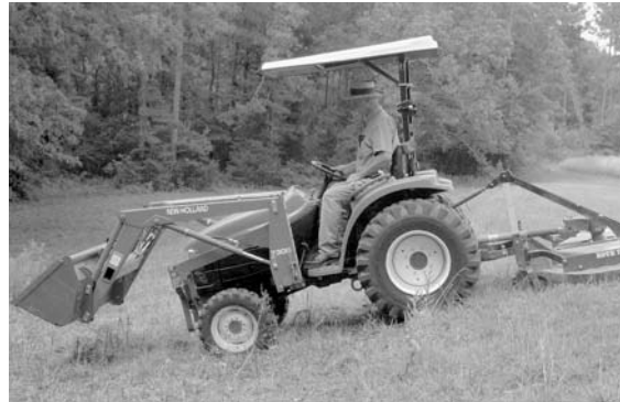
A tractor equipped with ROPS, seatbelt, and front wheel assist is safer to operate
