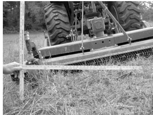
Yardsticks show the proper 3:1 slope of a levee to reduce tractor rollovers
