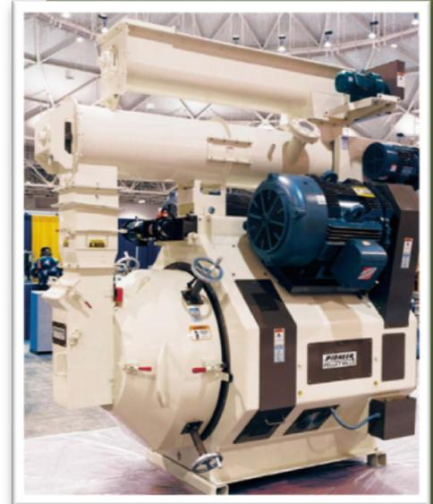
Large electric motors are used to power pellet mills, which compact wood particles and extrude them as pellets through small openings in steel dies.
