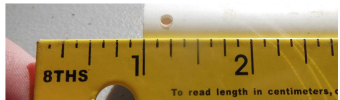
Figure 3.13. Drill the weep hole.
