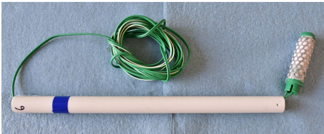
Figure 3.15. Thread the sensor wires through the PVC section.
