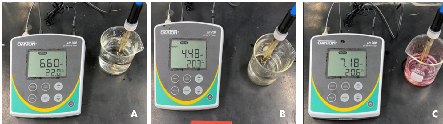
Figure 2. pH values for (A) tap water, (B) glyphosate solution, and (C) glufosinate solution.
