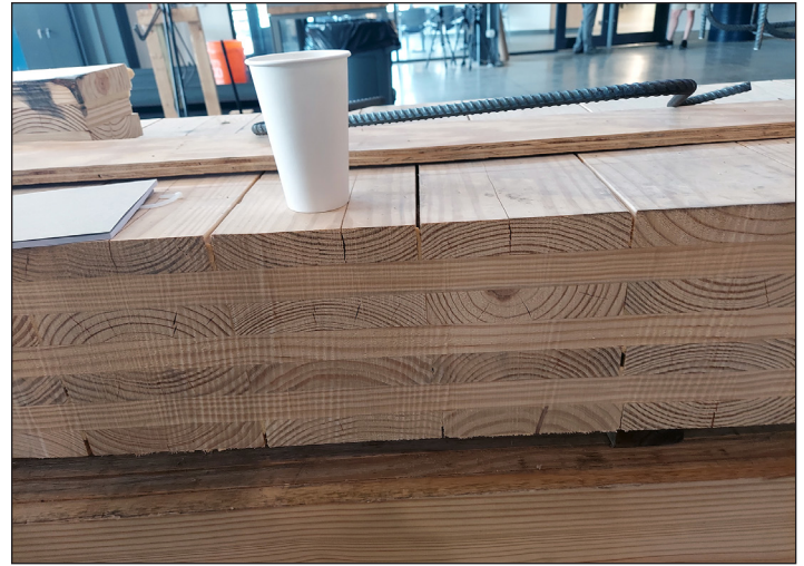
Figure 2. These are examples of a five-layer/ply piece (left photo) and a seven-layer/ply piece of cross-laminated timber (right photo). Notice the cross-directional, 90-degree joining of the layers/plies. For the seven-layer/ply picture, the cup provides a reference to demonstrate the thickness of the CLT piece.
