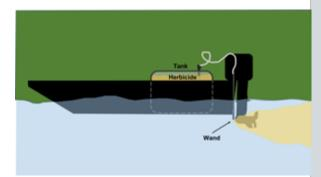
Herbicide injection uses the boat's motor to spread and mix the chemical in the water column. For application in deeper areas, weighted hoses can be used.
