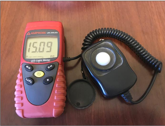
Figure 1. LED light meter used to measure light level.
