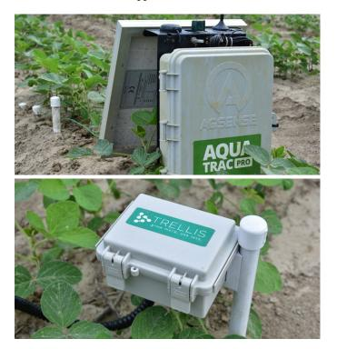
In some systems, each telemetry unit transmits its data independently over a cellular network. In other systems, multiple nearby "nodes" communicate via radio with the same base station, which transmits the collected data over a cellular network.
