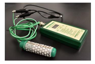
For convenient access, the pair of original sensor wires can be spliced to a pair of extension wires that run along the crop row out to one end of the field. To avoid affecting the readings, the manufacturer recommends using waterproof direct-bury splice kits and underground feeder (UF) wire that is 18 AWG for lengths up to 1,000 feet, 16 AWG for lengths up to 2,000 feet, and 14 AWG for lengths up to 3,000 feet.
