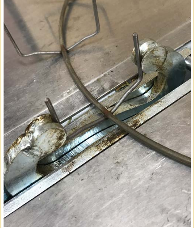
Figure 2. The clamp mechanism pinches heavy-gauge wreath wires around a gathered bunch of plant material stems.
