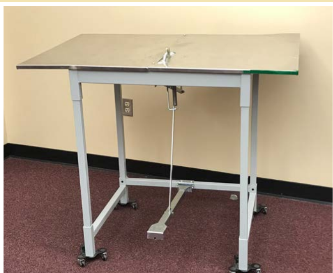
Figure 3. A pedal-operated clamp mechanism attached to a work table is a best practice for commercial producers.
