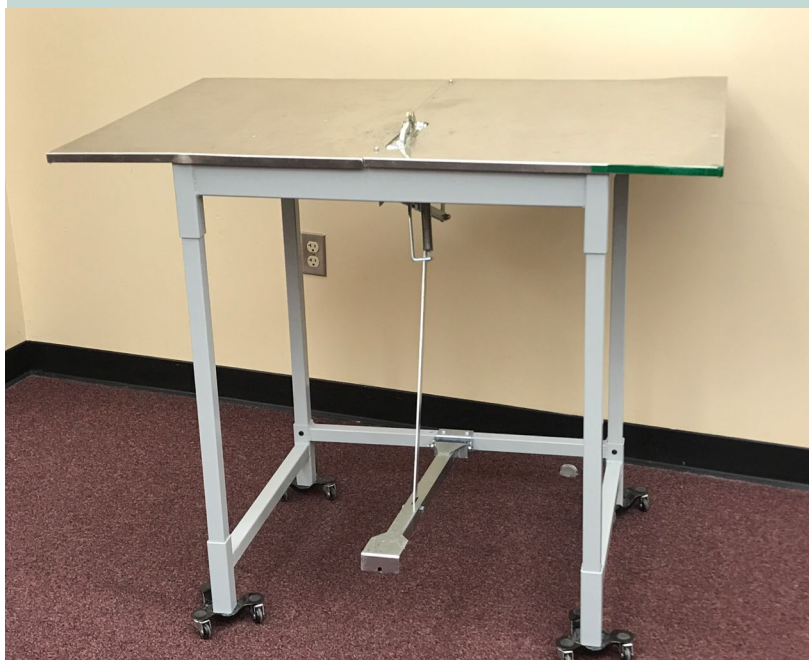
Figure 3. A pedal-operated clamp mechanism attached to a work table is the best practice for commercial producers.
