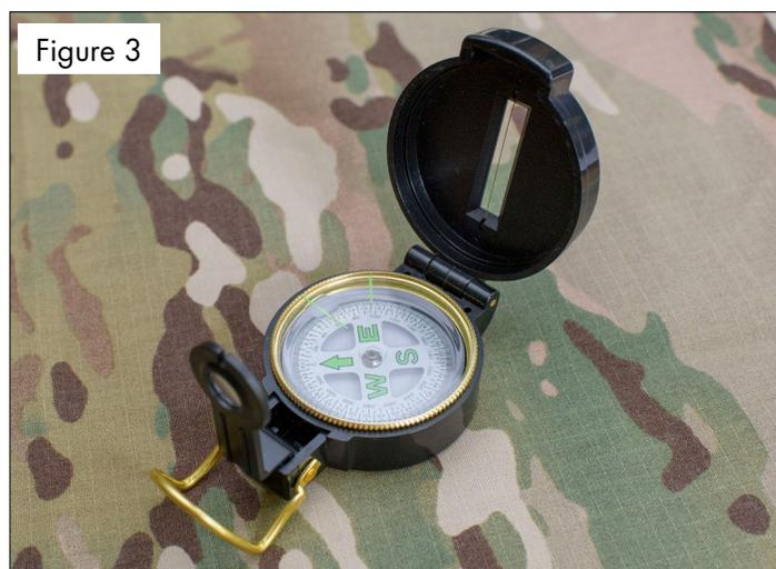
A commercial compass may have other components, too. Not only will one end of the needle be identified as north (or N) and the other south (or S), but typically east and west are identified, as well. A *lensatic compass* allows the user to get a fixed position on a distant object (**Figure 4**) and then determine the *degrees* in which that object is
