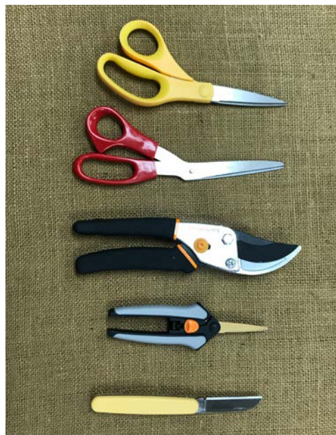
Figure 3. Cutting tools: multi-purpose, serrated-edge shears; scissors; pruners; floral snips; floral knife.
