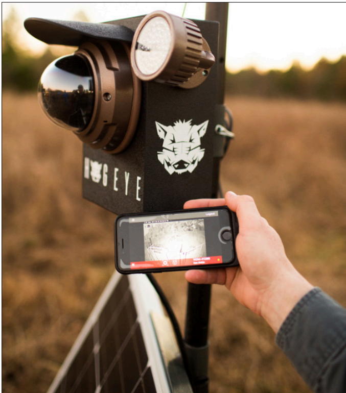
FIGURE 6. HOG EYE TRAP CAMERA AND MOBILE APP USED TO CATCH FERAL HOGS.
