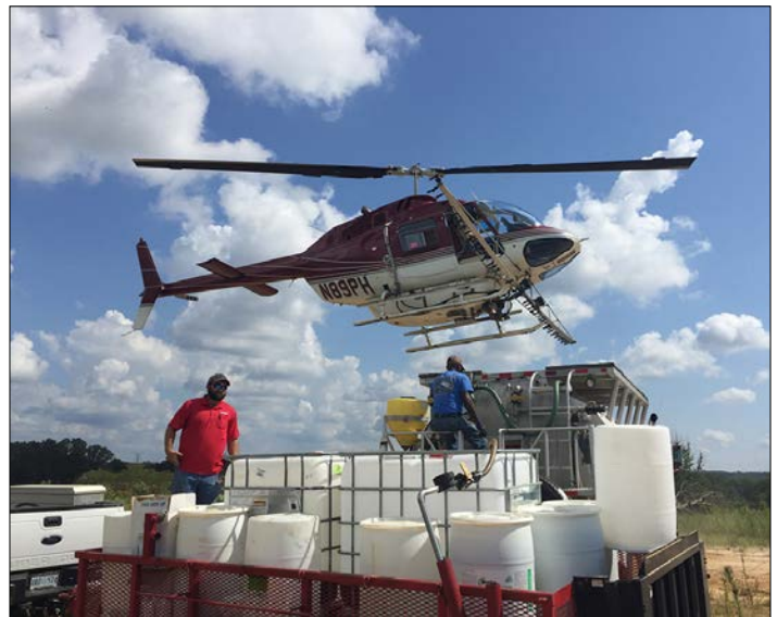
Figure 5. Helicopter refilling with herbicides during a site preparation application. Photo by Brady Self.
