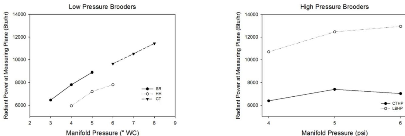
Figure 4. Effect of varying manifold pressure on total radiant power at the measuring plane of low- and high-pressure round radiant brooders. The middle point in each line graph represents the rated manifold pressure for the respective brooder.
