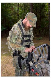
Whether the stand is new or old, it needs to be inspected periodically. Check for parts that may be loose and straps and cables that need to be replaced. Stands that have been left outside since the previous season pose a significant danger. Always check welds and connection points (screws and pins) to make sure they are not broken or loose. If you have a wooden stand, shake it and inspect it
