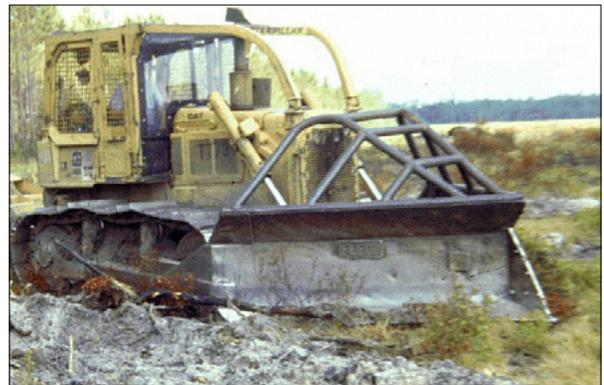
Figure 2. Land-clearing involves shearing large material with a tractor-mounted blade or by hand using a chain saw.
