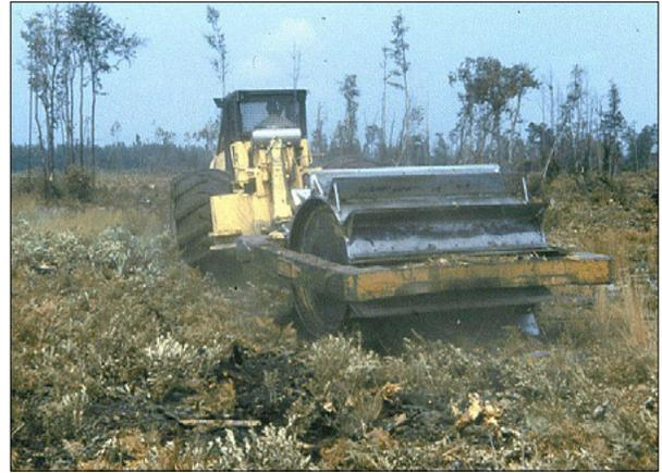
Figure 4. Smaller residuals are cut into pieces by a rolling drum chopper. The drum can be filled with water to add weight. A prescribed burn can then be done to reduce the amount of residuals before planting.
