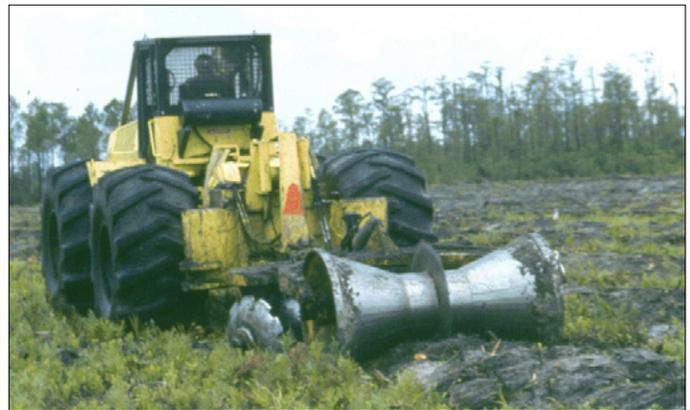
Figure 6. The bedding harrow cuts and mounds the soil into a planting row for enhanced drainage on wet sites.
