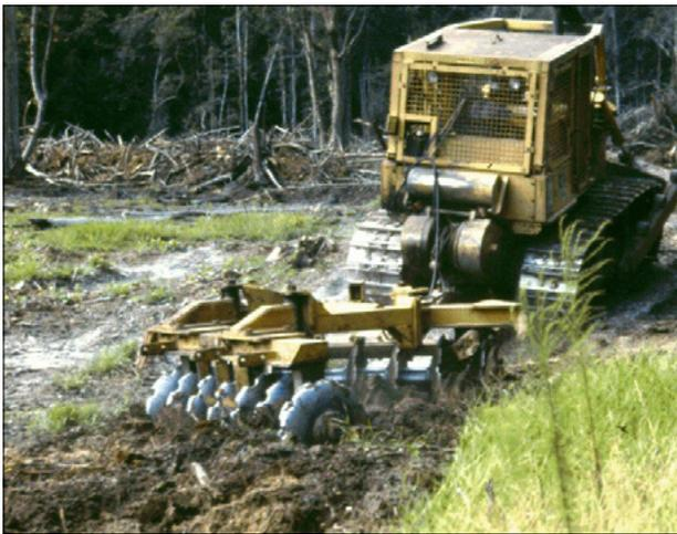
Figure 5. Disking with an offset harrow controls competing vegetation by cutting and exposing roots. Disking can also restore the site from rutting and compaction during logging and land-clearing.
