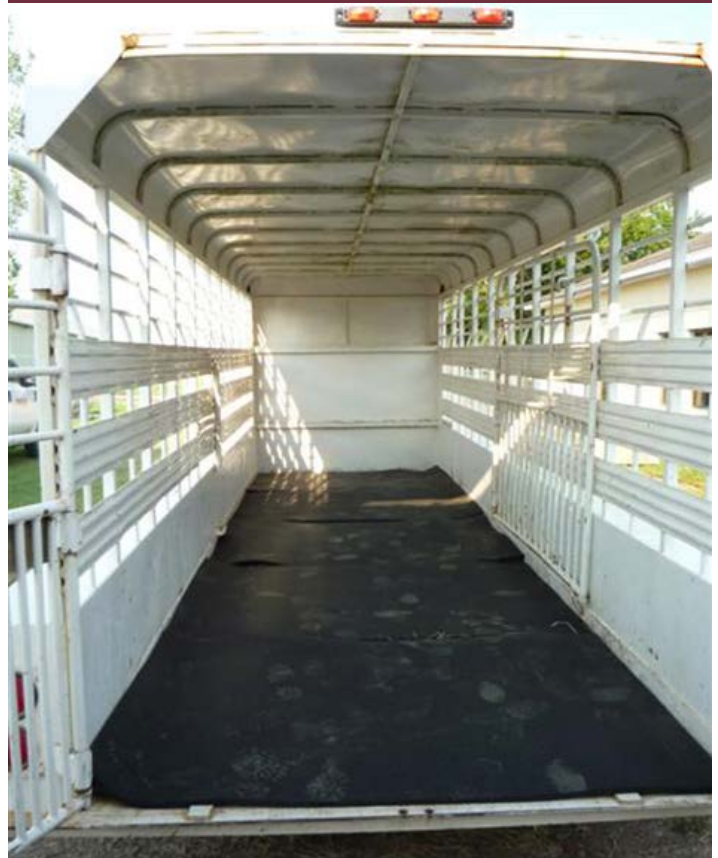
Figure 2. Rubber mats improve traction on trailer flooring.
