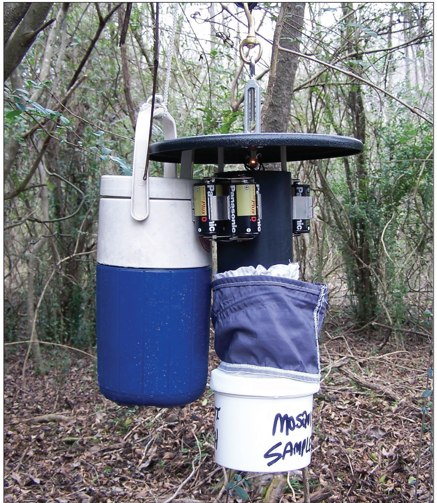
Figure 4. CDC light trap with dry ice as a carbon dioxide source
