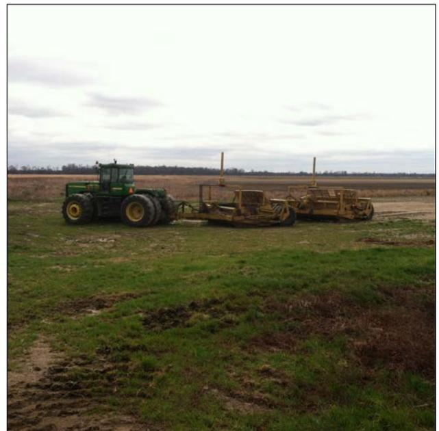
Figure 4. Tractor and dirt pan used to move soil to level land, as well as create TWR ditches and OFS reservoirs.
