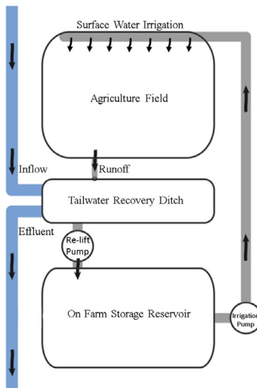
Figure 2. Diagram of a generic TWR system. Not all TWR systems are designed the same as this diagram. Some TWR systems do not require an extra on-farm storage (OFS) reservoir, and most of them collect water from multiple fields. Source: Omer et al. (in press a).
