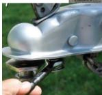
Connect trailer electrical plug and breakaway cable to vehicle; ensure all lights work & brakes are adjusted correctly.
